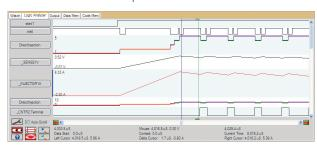
When using graphical state machine development, view states as a color-coded, vertically-keyed, enumeration. Vertical cursors can snap to the state transitions and the cursor time can be dropped into the simulation thereby resetting simulation to the start of the snapped-state.
