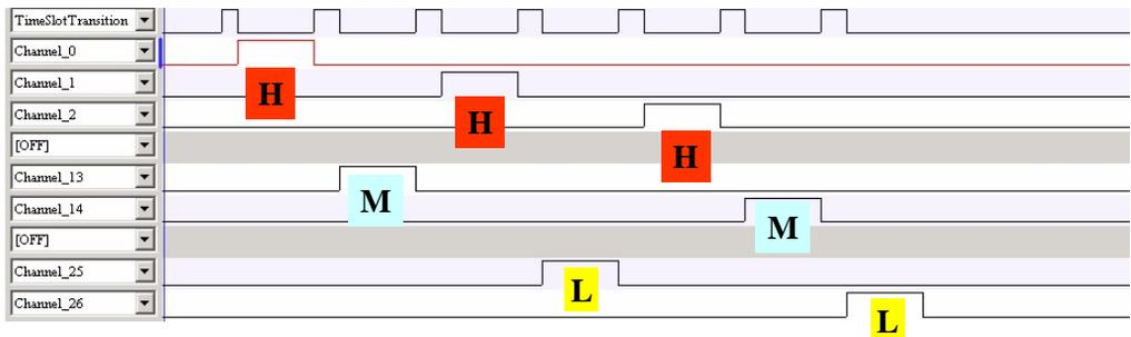
As can be seen in the above diagram, within the High priority group, channel 0 gets schedule before both channel 1 and 2 because '0' is less than '1' and '2'. Similarly, within the Middle priority group, channel 13 is schedule prior to channel 14, and within the Low priority group channel 25 is schedule prior to 26.
