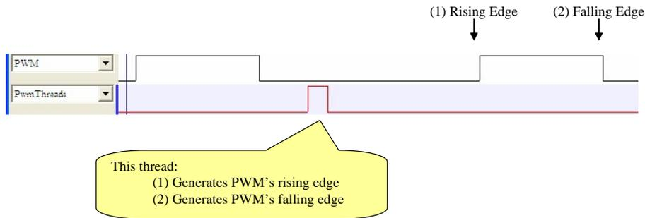
Since the thread contains two tasks (generate rising and falling edges) it will be broken into two smaller threads that each do one of these tasks. In this case the following approach will be taken.
