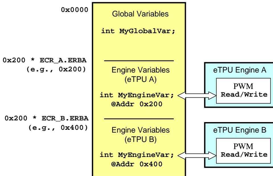
A significant drawback of using engine-relative base address register is its granularity which is `0x200` bytes. This can lead to significant RAM wastage. The true (byte) address of any access is calculated as follows
