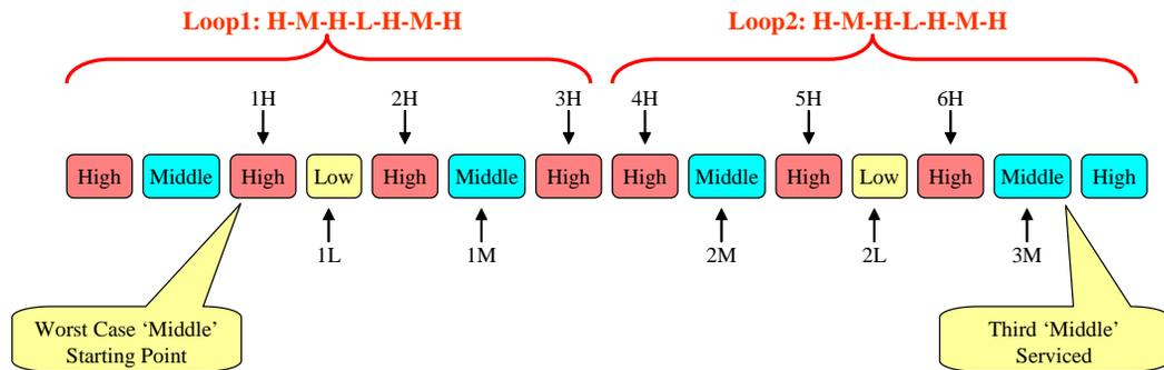
As seen in the above diagram, there are 6 High priority time slots, 3 Middle priority time slots, and 2 Low priority time slots between when the Middle channel seen to the left of the 'Worst Case Middle Starting Point' and when that same Middle priority channel completes its second servicing indicated in the above diagram as 'Third Middle Serviced' channel.
