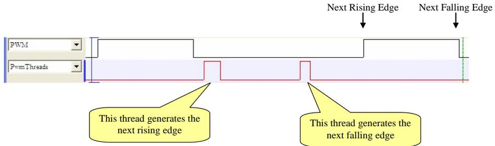
The sequence events from the falling edge that generates the second thread is as follows.
