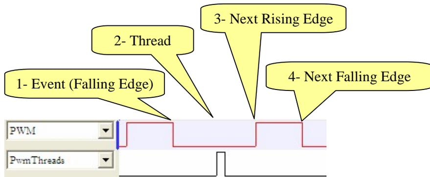
In the above diagram, if the thread (2) should become so delayed that it occurs later than when the next rising edge (3) is supposed to occur, then the next rising edge (3) will be either delayed or missed entirely. The exact behavior depends on how the channel is configured (this will be covered later) but for now assume that neither scenario (PWM operation ceases or lag in the PWM signal) is particularly desirable.
