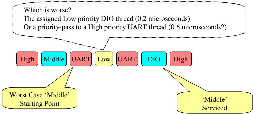
So by priority passing, in this simple case with only three active channels (one at each priority level) the middle priority WCL increases due to priority passing from the (shorter) low-priority time slot thread to the longer high-priority time-slot thread.
