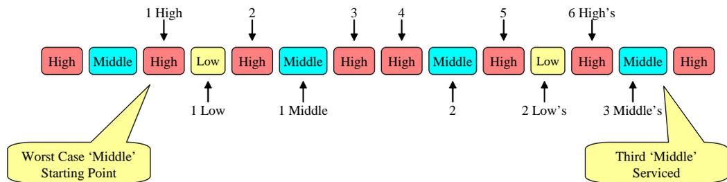
In the above example, the WCL contributors are 6 High priority time slots, 2 Low priority time slots, and 3 middle priority time slots for a total of 11 time slots. The Time slot of each Middle priority channel represents just 1/11 of all the time slots that contribute it its WCL.
