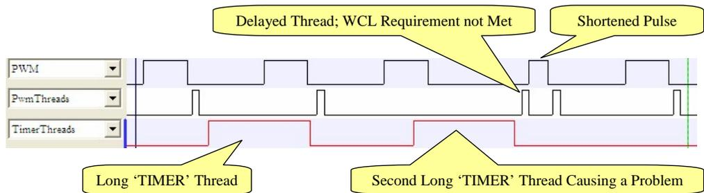
However, if the MATCH comparator has been configured in 'Equals Only' mode then the TCR1 (or TCR2) counter must complete a full cycle and return to 20 before the output pin's rising edge is triggered. If the MATCH is triggered off a free-running TCR1 counter, the best case rollover is around 250 milliseconds, which is an electronic eternity.
