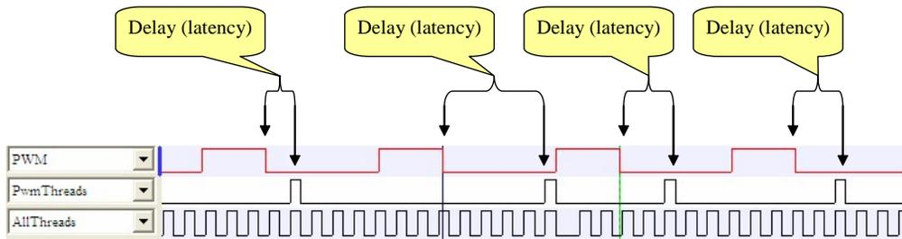
The delays vary because the number of other channels requesting servicing varies. For instance the first delay seen above is quite a bit shorter than the other delays, and the second delay is quite a bit longer than the others. In fact, the second delay is so long that the PWM is in risk of not functioning properly.
