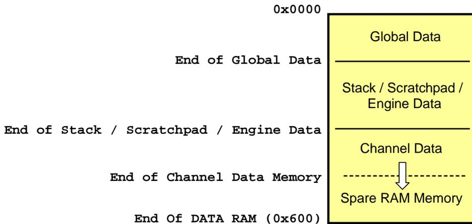
The memory layout listed above is supported by the many #defines that are automatically generated by the linker. These #defines are found in the auto-defines file which is the same as the output ELF/DWARF file (unless overridden or disabled) except that the file suffix (.ELF) is replaced with ‘\_defines.h’.
