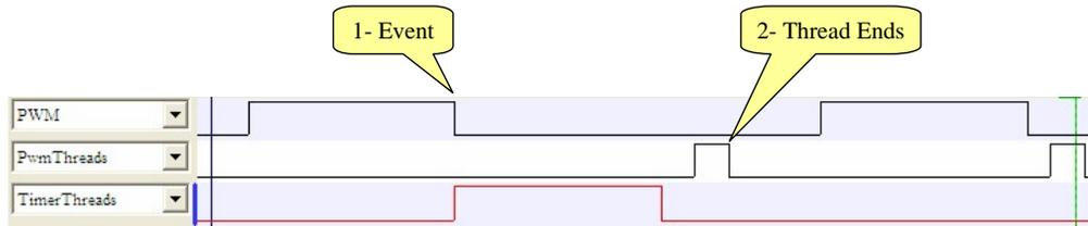
In this simple example at the exact moment the PWM thread would be scheduled, a TIMER thread gets scheduled first such that the PWM thread must wait until the TIMER thread completes. There is an additional short delay between when the TIMER thread ends and the PWM thread begins known as a ‘Time Slot Transition’ or TST. The TST typically lasts 6 system clocks and is required by the scheduler to decide which channel to schedule for servicing next and to prepare the next thread for execution.
