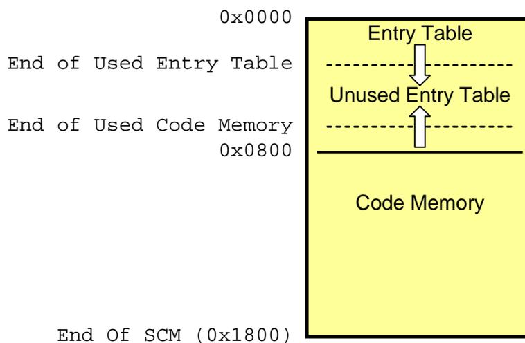
The entry table is effectively an array of thread-start address pointers. Unused entry table is filled with pointers to the Error Handler Library. This allows observability of accidental access of entry table because the corresponding bit in the `_Global_error_data` gets set.
