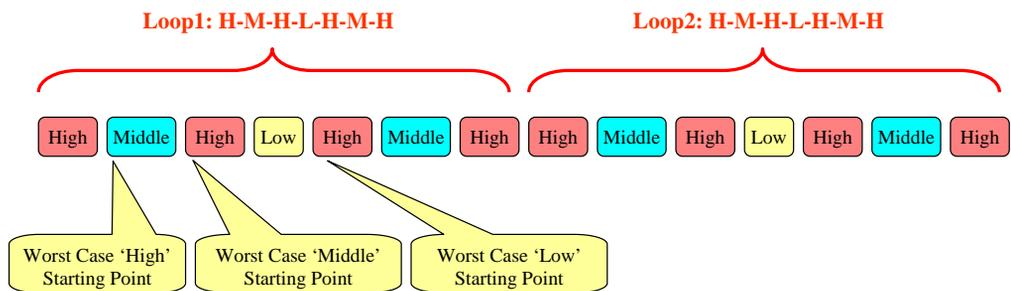
To determine the WCL at each Priority group of channels, start with the worst-case time slot shown above and progress forward until all channels of that time priority level have been serviced once. Add up the number of time slots of each priority group.
