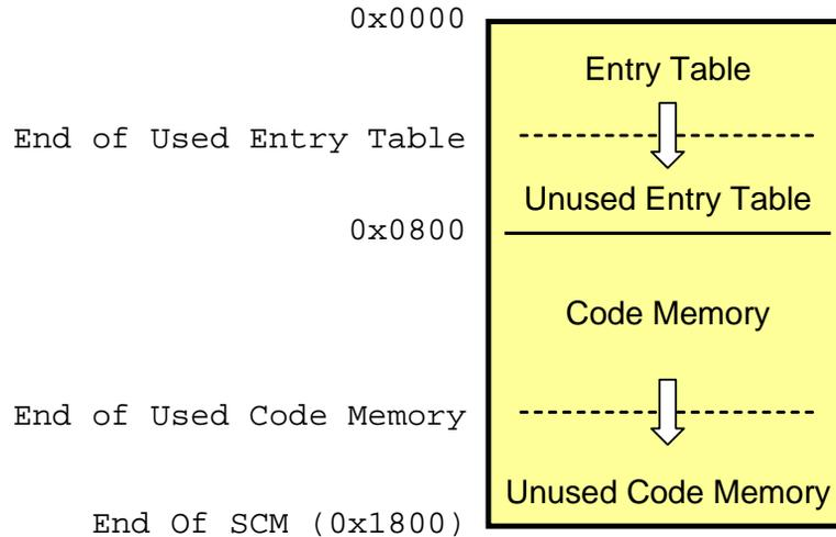
As seen in the above diagram, the entry table base defaults to address zero. As eTPU Functions and eTPU Classes are added, they are fill towards address 0x800.
