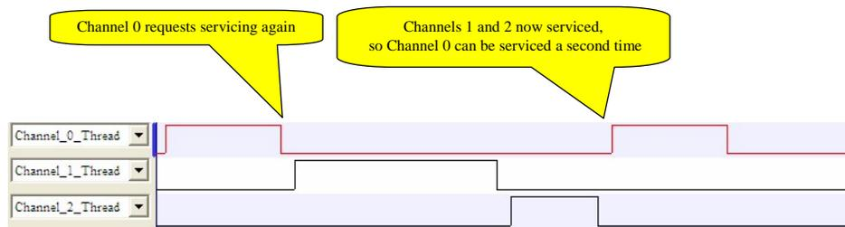
As seen in the above diagram, the tertiary priory scheme prevents channel 0 from getting serviced a second time until both channels 1 and 2 have been serviced. This prevents lockout on channels 1 and 2.
