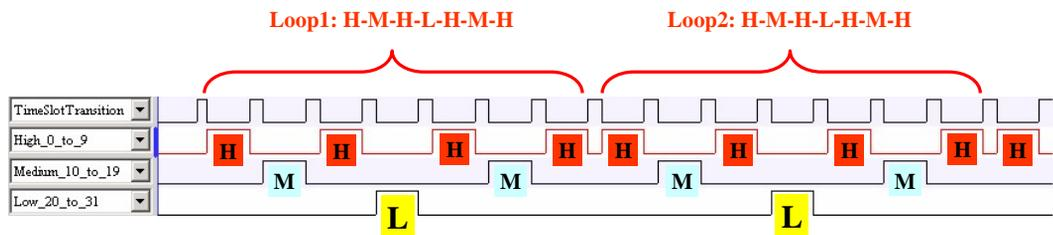
As can be seen in the above diagram, some Middle and Low priority channels do get scheduled before some High priority channels so what exactly does the priority level mean? Notice that at the end of the second loop, eight High priority channels have gotten
